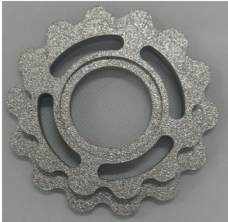
Fig.15. A compound of lobe-cams after PBF machining processes
