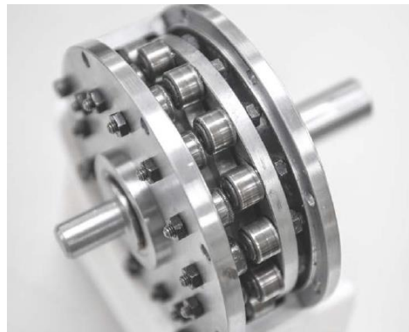
Fig.11. A lobe-cam reducer
