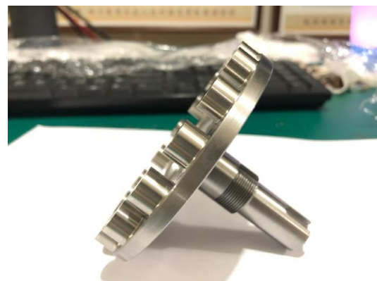
Fig.13. A roller disc after DED machining processes
