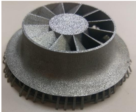
Fig.16. A shrouded centrifugal impeller after PBF machining processes
