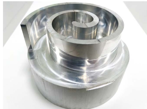
Fig.19. Scroll workpiece after semi- and fine machining processes
