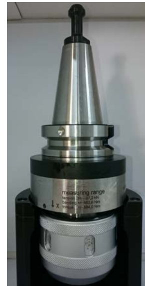
Fig.8. Tool holder with sensors
