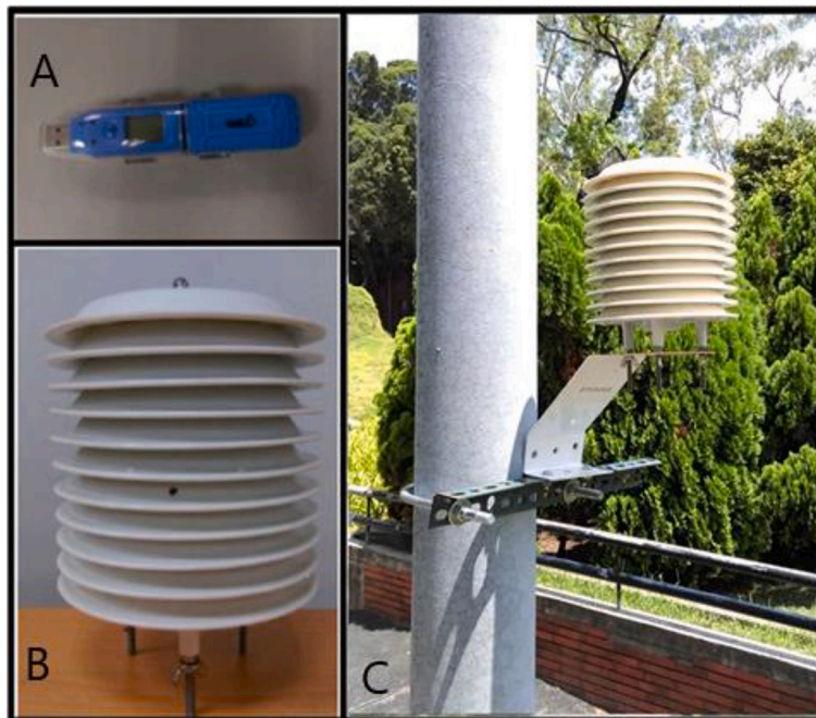
Fig. 2. Equipment installed at a measurement point. (A) LOGPRO instrument. (B) Radiation shield. (C) LOGPRO instrument and radiation cover at a measurement point.
