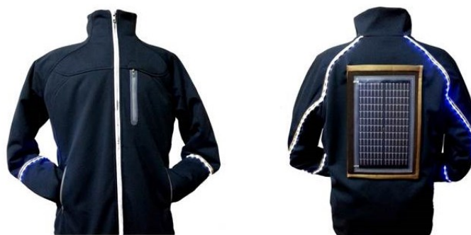
Fig. 3 A multifunctional jacket with optoelectronic components: front and back sides
